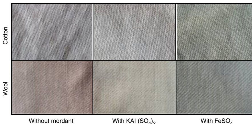
Figure 3 Colours obtained on cotton and wool by using nutshell as a natural dye [Colour figure can be viewed at wileyonlinelibrary.com]
